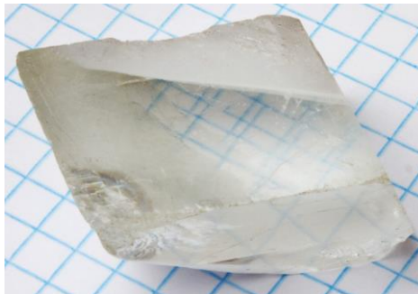
Figure 9. A calcite crystal displays the double refractive properties positioned on a sheet of graph paper. (APN MJM, 2/6/2012 via Wikimedia Commons, Creative Commons Attribution)
