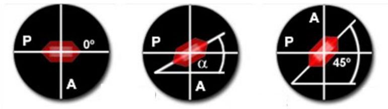
Figure 17. The light intensity crossing a system composed of two crossed polarizers with a sample of birefringent material in between varies when rotating the sample. (Image adapted from Murphy et. al. (ref. 20))
