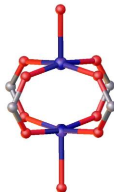
Figure 3. Copper (blue) square paddle-wheel SBU. Oxygen atoms are in red while carbon is displayed in grey (Bosch M. et al., Advances in Chemistry , 2014 , ID 18232).
