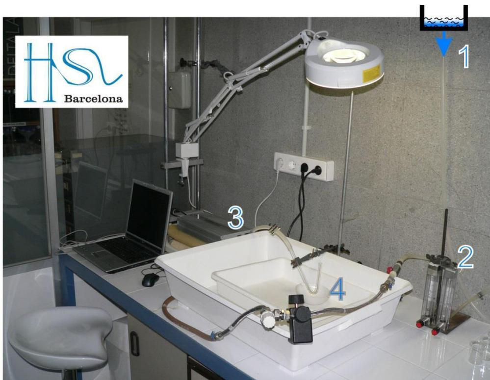
**Fig. 3.1.** Hydroseparation laboratory Barcelona ([www.hslab-barcelona.com](http://www.hslab-barcelona.com)); 1 water tank; 2 flowmeters; 3 software controlled HS-11 device; 4 Glass Separation Tubes (GST).
