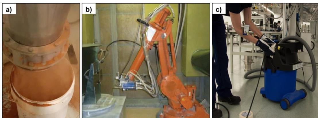
Figure 1.4 Industrial processes with potential to generate nanoparticles in workplace air: a) ceramic milling processes; b) atmospheric plasma spraying; c) use of vacuum cleaner.
