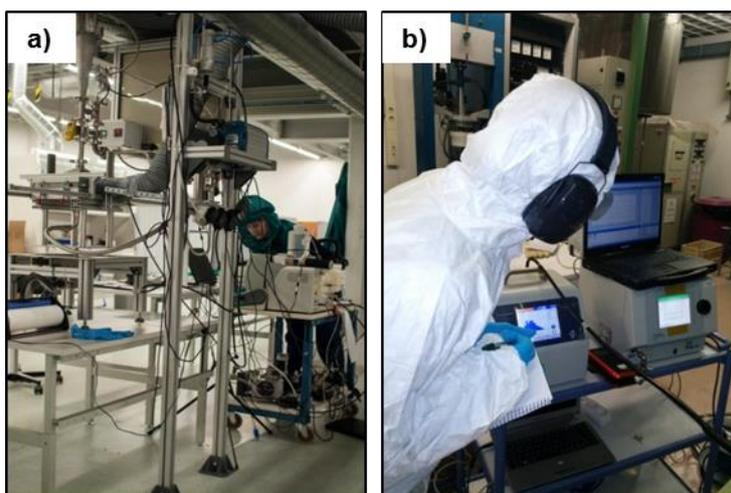
Figure 1.10 Well protected researchers assessing occupational exposure to nanoparticles during: a) SWCNT manufacturing, and b) atmospheric plasma spraying applied in ceramic industry.
