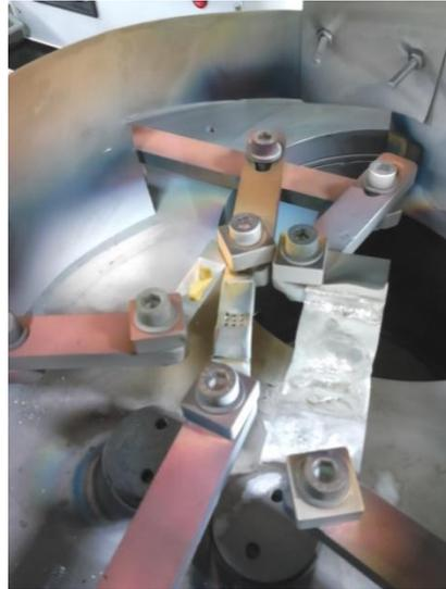
Figure 6.1: Base holders inside the vapor deposition chamber, where the different metals are placed for evaporation. From left to right the holder for Au, Cr and Al.
