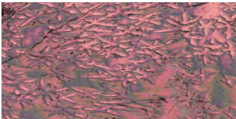
*Figure 4.3-1: Image of the optical microscope coupled to the Raman spectrometer where we can see the 4-lobes and 6-lobes graphene domains. The image corresponds to domains that have been transferred over SiO<sub>2</sub>. (Sample 15C2001)*
