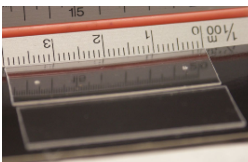
Fig 2. Two PMMA pieces with one side drilled with 2 x 1 mm holes.
