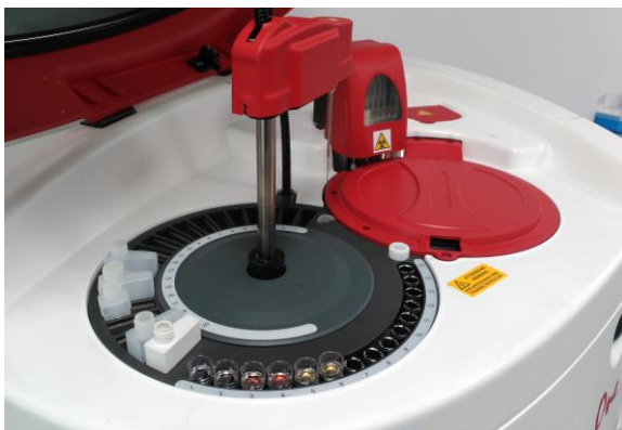
Figure 8. Miura One®'s interior. Rotary sampling arm, reagents' and samples' positions, rotary cuvettes system (red circle).
