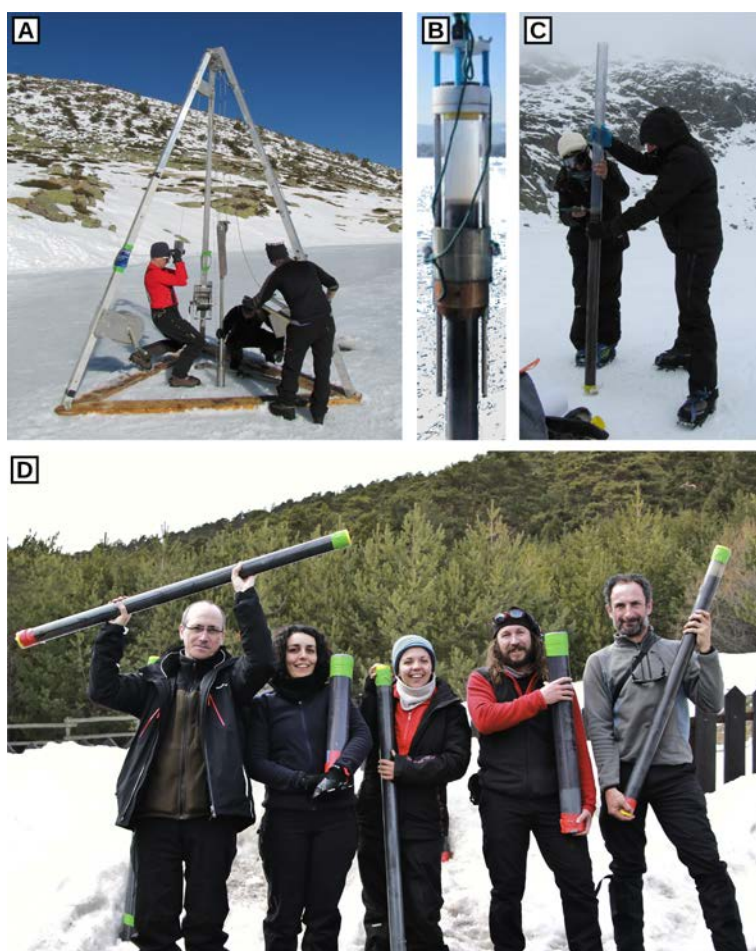
Figure 3.5. UWITEC ® A) piston and B) gravity recovering systems. C) Cutting a sediment core recovered from Cimera Lake in March 2012 before to be sealed the core with foam. D) Sediment cores recovered from Peñalara Lake in February 2012.
