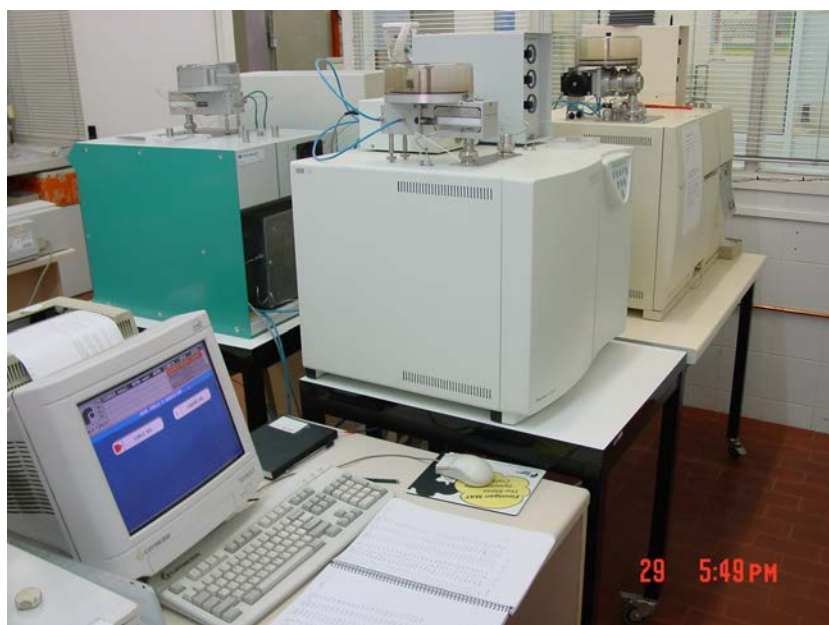
Figure 3.14. Image of the Finnigan DELTAplus® TC/EA-CF-IRMS spectrometer at the CCiT-UB (Barcelona, Spain) (photo by J.J. Pueyo).
