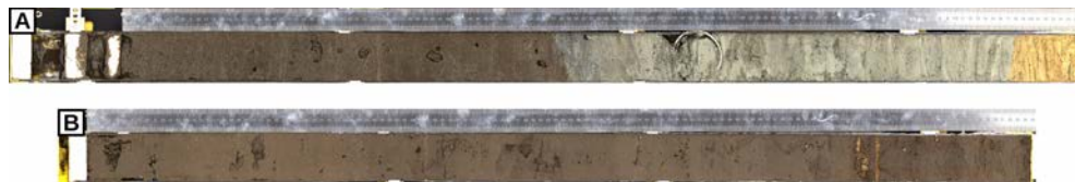
Figure 3.7. Core images acquired with a colour line-scan camera of A) the PE-12-01-01 core from Peñalara Lake and B) the CIM12-04A core from Cimera Lake. Top of both cores on the left.
