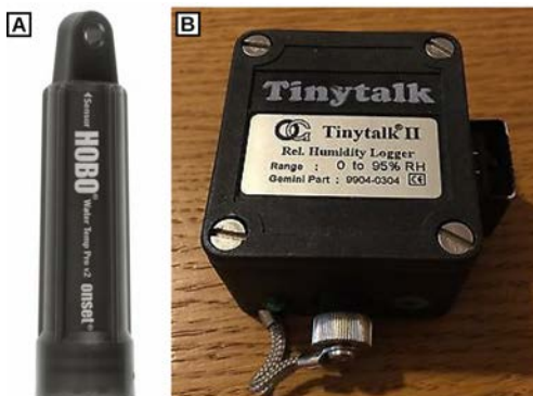
Figure 3.3. Photos of A) HOBO Water Temp Pro V2 and B) Tinytalk II thermistors.
