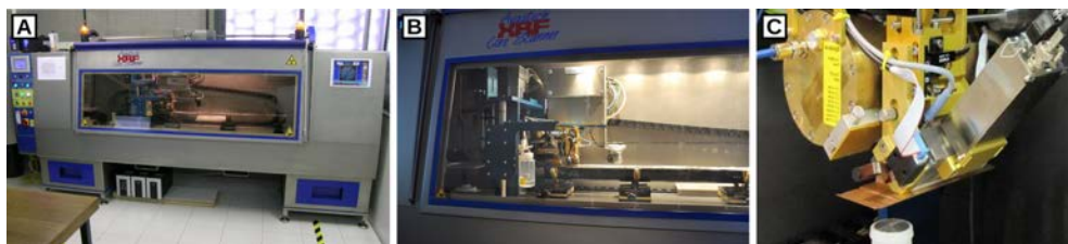
Figure 3.10. A) Image of the XRF Avaatech core scanner at the University of Barcelona (Spain). B) XRF Avaatech core scanner measurement system moving along a core half. C) The prism of the XRF Avaatech core scanner measurement system (photos by J. Frigola)
