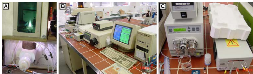
Figure 3.15. A) Plasma source of the inductively coupled plasma mass spectrometer (ICP-MS) and B) ion chromatography line, both at the CCiT-UB (Barcelona, Spain). C) A detail of its column and injection pump.
