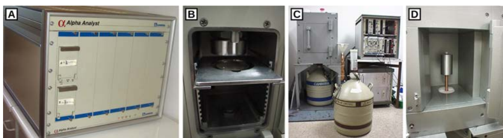
Figure 3.9. A) ORTEC® and B) Canberra® alpha spectrometers used for the ^{210}\text{Pb} analyses. C) HPGe gamma spectrometer and its D) coaxial Ge detector used for the ^{226}\text{Ra} and ^{137}\text{Cs} analyses. All the equipment is located in the LaRAM ICTA-UAB (Barcelona, Spain). Photos by J.J. Bruach.
