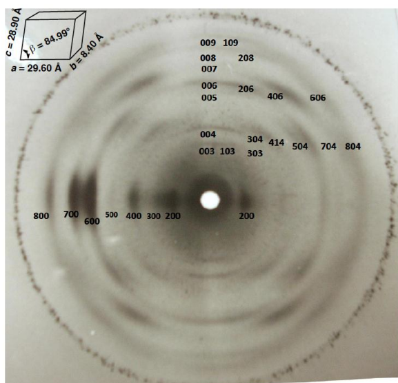
Figure 1. X-ray diffraction image of H_4TPPS_4 J-aggregates and inferred unit cell dimensions (space group P2_1 with four porphyrins in the unit cell); h,k,l parameters for strong, medium, weak and broad spots are shown. The outside ring is the distance control (powder silicon standard, 3.1355 Å). For the comparison of experimental vs calculated distances see Table in Supplementary Information.
