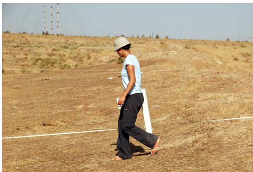
Fig. 5: Surveying with the magnetic gradiometer
