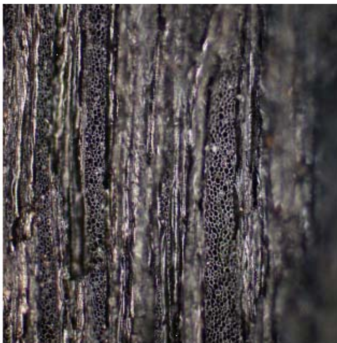
Figure 4. Tangential longitudinal section of Platanus sp
