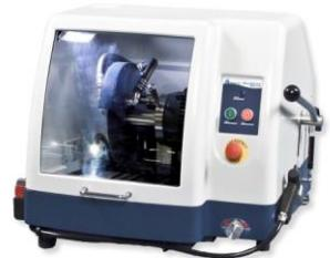
**Figure 5.5.**Image of abrasive cutter
