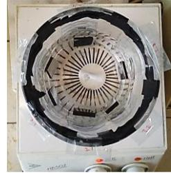
Figure 5.15. Flooding corrosion device
