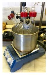
Figure 5. Distilling flask in oil bath
