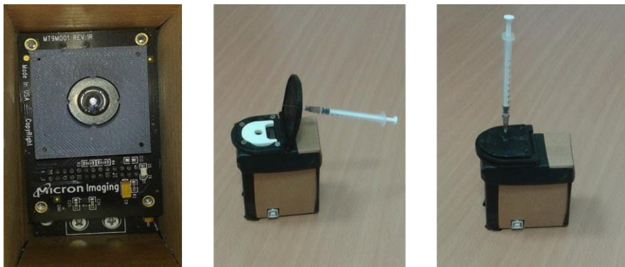
Figure 5.7 From left to right: CMOS camera in the device structure, opened device with the holder inside and device ready for the assay.
