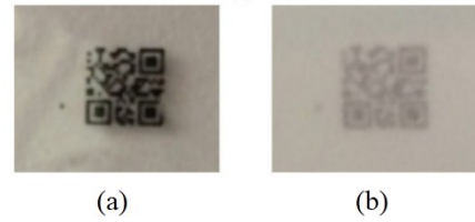
Fig. 2. (a) Experimental 4 mm × 4 mm QR code and a picture of (b) 3D optical phase code A, which consists of a QR code with an optical phase mask consisting of a glass slide and diffuser paper.
