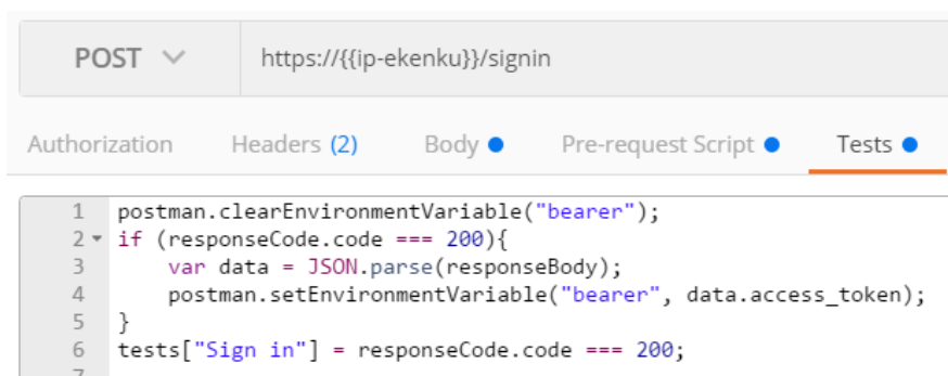
Figure 35. Post request script, saving data needed for authentication
