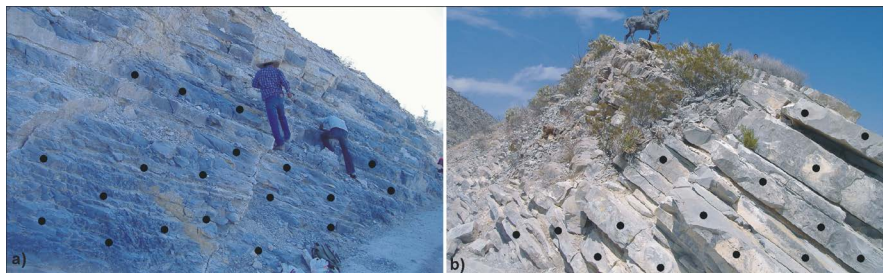
Figure 3. Outcrops of carbonated rocks. (a) Aurora Fm; (b) Washita Group. Filled black circles indicate measurements points in the outcrops.
