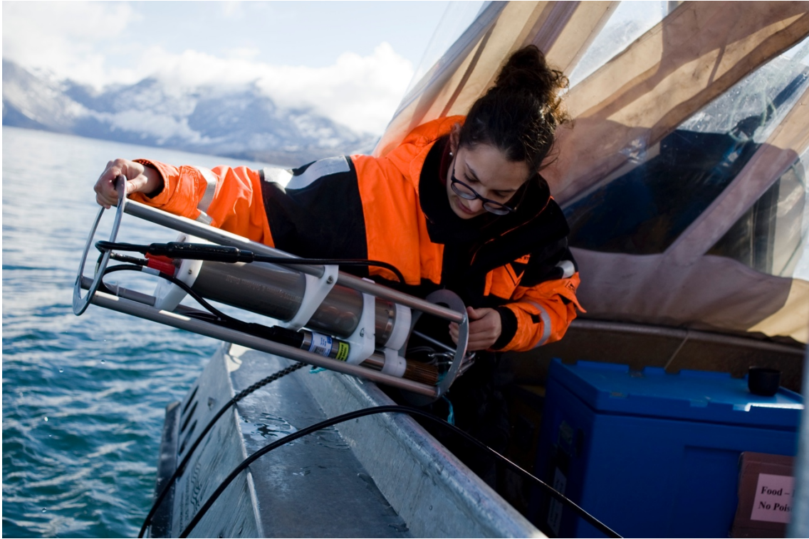
Image 5: Deployment of the equipment to measure p\text{CO}_2 in the water column aboard the Erissalikk boat in Godthåbsfjord, Greenland. Photo credit: F. Ugarte.
