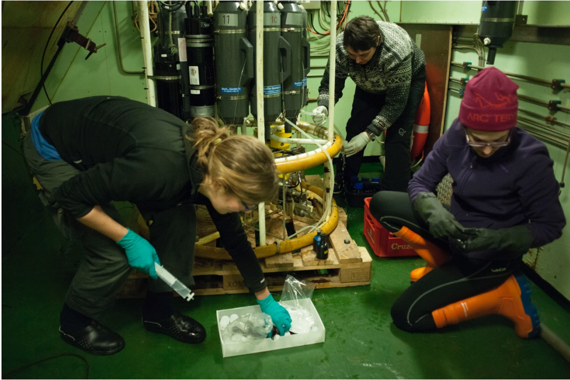
Image 4: Seawater sampling from a rosette system fitted with Niskin bottles aboard the R/V Helmer Hansen. Photo credit: R. Caeyers.
