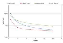
**<u>Figure 7.</u>** Viscosity of monomodal emulsion  $d(0.5)_{p}$ monomodal emulsion  $d(0.5)_{s}$ , and bimodal emulsion with 80% residual bitumen
