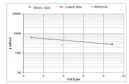
**Figure 8.** Viscosity as function of the droplet size for a monomodal emulsion  $d(0.5)_p$  monomodal emulsion  $d(0.5)_s$  and bimodal emulsion with 80% residual bitumen
