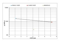
Figure 6. Viscosity of monomodal emulsions (large and small size) and bimodal emulsion as function of diameter size
