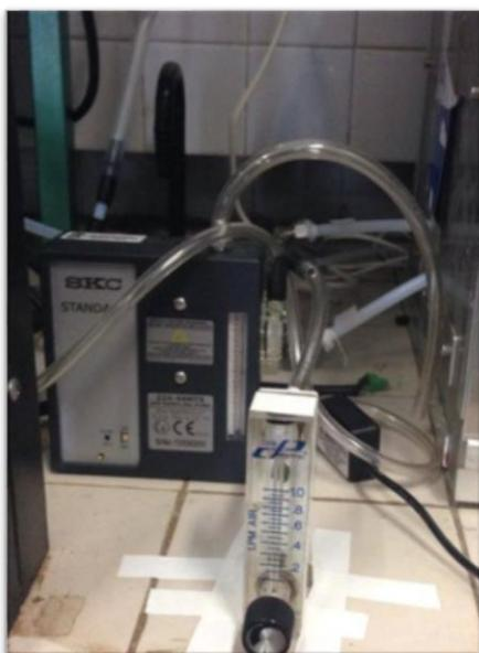
Figure A.10. Sampling pump with rotameter
