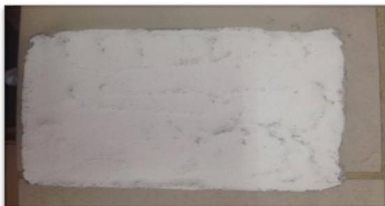
**Figure 4.2.** Mortar of cement with 5% concentration of  $\text{TiO}_2$ .
