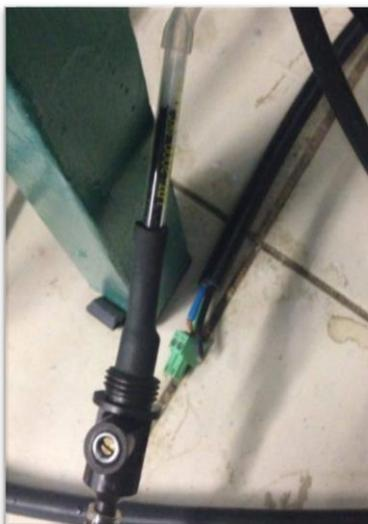
**Figure A.8.** Sampling pump with activated carbon tube
