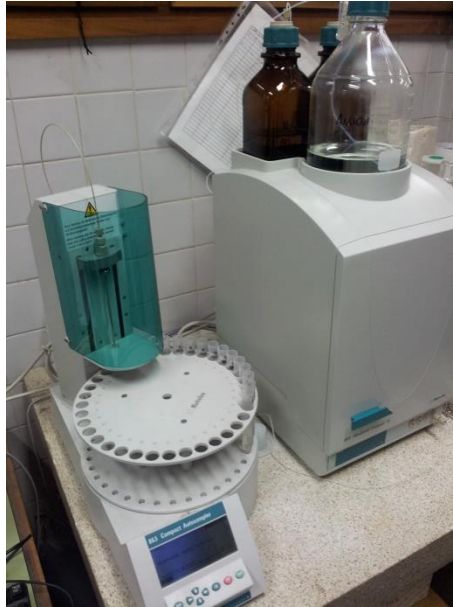
Figure 4: Ionic chromatograph, Metrohm 861 Advanced Compact IC and its autosampler
