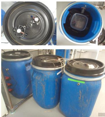
FIGURE 6 DYNAMIC CHAMBER CONSTRUCION (DRUM 1: CONTROL (WIHOUT VENTILATION); DRUM 2: 2 FANS OF 12V; DRUM 3: 1 FAN OF 12V
