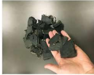
Input: Tire Shreds smaller than 200 mm (8"-inch) minus.
