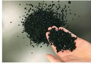
Output: 16 - 4 mm (0.625" - 0.16" -inch) and smaller crumb rubber
