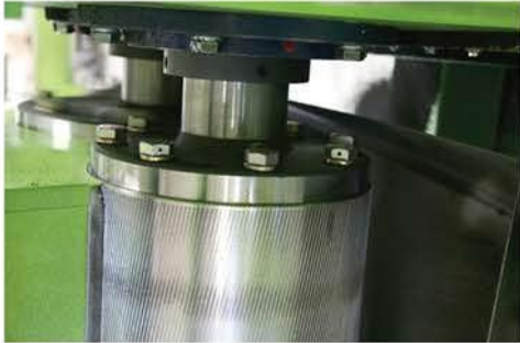
Multiple Roll Corrugations Available Sealed, Low Grease Bearings
