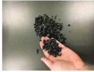
Output: 38 - 16 mm (1.50" - 0.625"-inch) and wire-free rubber mulch/chips.
