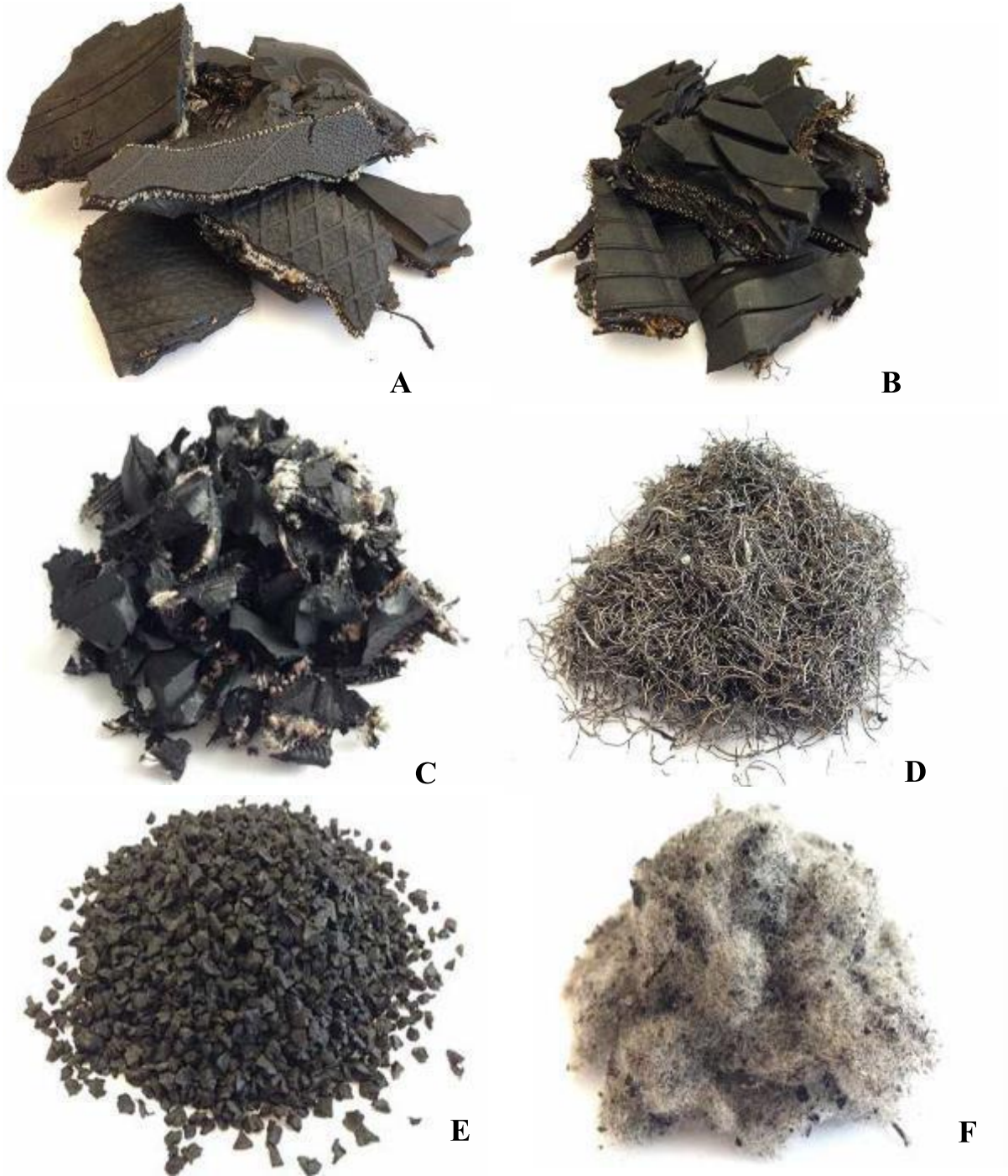
(A) Tyre Shreds (~150 mm), (B) Tyre Chips (~50 mm); (C) Wire-Free Rubber Chips (~38-16mm), (D) Steel Wire, (E) Granulate Rubber (~16-4mm and smaller) and (F) Liberated Textile fiber.
