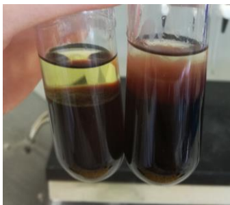
Figure 2. Beans extract with NaCl (left) and without NaCl (right). Both with 1 g of broad beans, 10 mL saponification solution and 5 mL of hexane.
