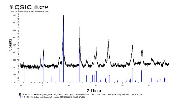
Figure S1. Powder X-ray diffraction scan from dense abellaite aggregates. For comparison, the X-ray diffraction pattern of synthetic NaPb<sub>2</sub>(CO<sub>3</sub>)<sub>2</sub>(OH) from Brooker *et al.* (1983) is also shown.
