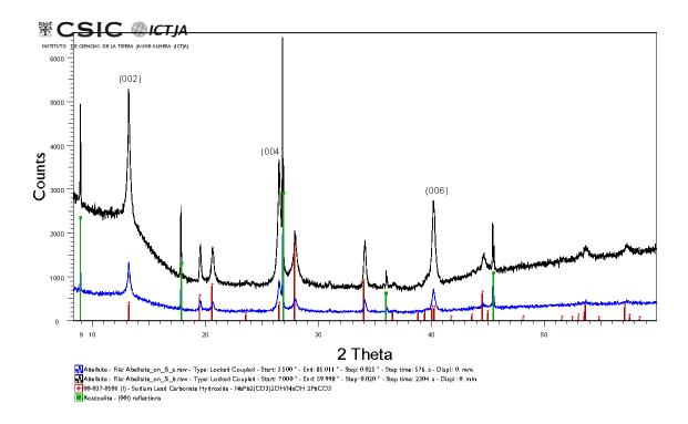
Figure S2. Powder X-ray diffraction scans of abellaite grains on a low-background Si sample holder. For comparison, X-ray diffraction pattern of synthetic NaPb<sub>2</sub>(CO<sub>3</sub>)<sub>2</sub>(OH) from Brooker *et al.* (1983) and roscoelite [only (00*l*) reflections] are included.
