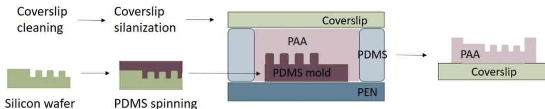
Fig. 3. Fabrication process of the PAA hydrogels
