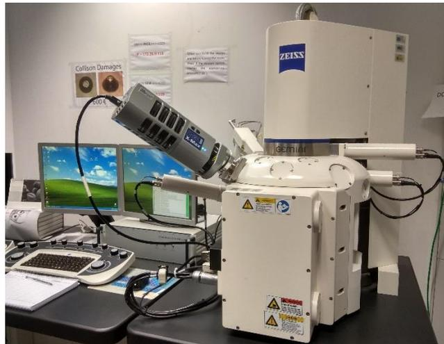
**Figure 2.19:** Scanning electron microscope coupled to EDX located at IREC.
