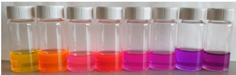
Figure 3. Solvatochromic behavior of Nile Red can be easily seen when it is dissolved in different solvents. From left to right: hexane, tert-butyl methyl ether, chloroform, acetone, ethanol, methanol, acetone-water (1:1) and water
