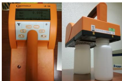
Figure 8. On the left, \beta/\gamma counts per second are shown in the GM screen. On the right, set up for crushed banana geometries measurement.
