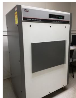
Figure 4. 1220 Quantulus liquid scintillation detector by EG&G Wallac.
