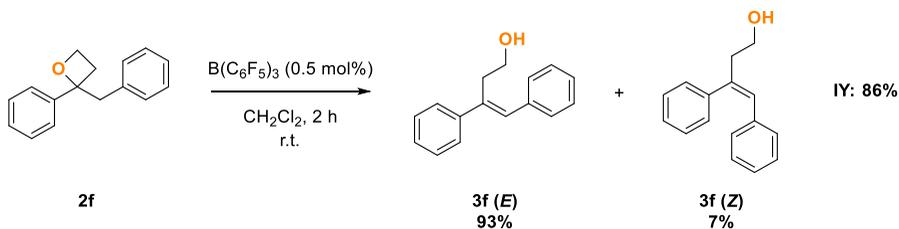
Figure 16: Isomerization of the benzyl substituted oxetane (**2f**) following GP 2
