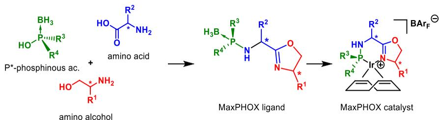
Figure 3: Synthetic scheme of Ir-MaxPHOX catalyst
