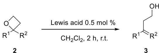
Figure 20: General scheme for the isomerization of the oxetanes to the homoallylic alcohol
