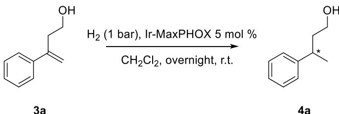
Figure 21: Scheme for the asymmetric hydrogenation of **3a** using Ir-MaxPHOX as the catalyst
