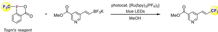
Scheme 6. Trifluoromethylation via photocatalytic decomposition
