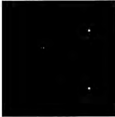
Figure 5.13- Pixel by pixel multiplication of the ten binarized correlations of Figure 5.12. A perfect detection of letters e and s is now possible.
