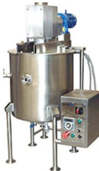
Figure 25: Example of closed stirred and jacketed tank for dissolution (25/08/2019, Tecnodac)
