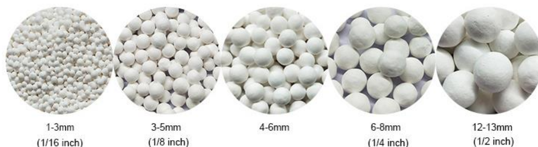
Figure 17: Example of sizes of alumina spheres.
