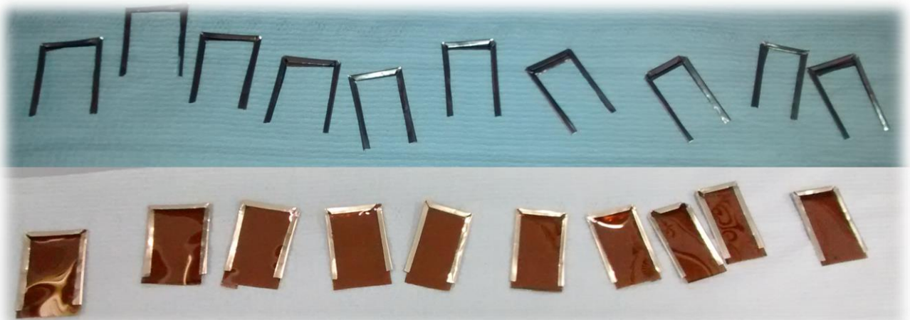
Figure 43. Homemade frames employed initially for polyimide substrate handling.
