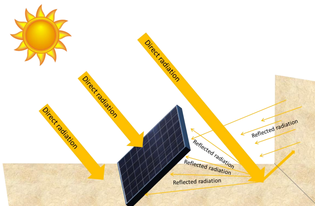
Figure 87. Schematic of albedo light reaching the front and rear sides of a bifacial solar panel in a rooftop installation.
