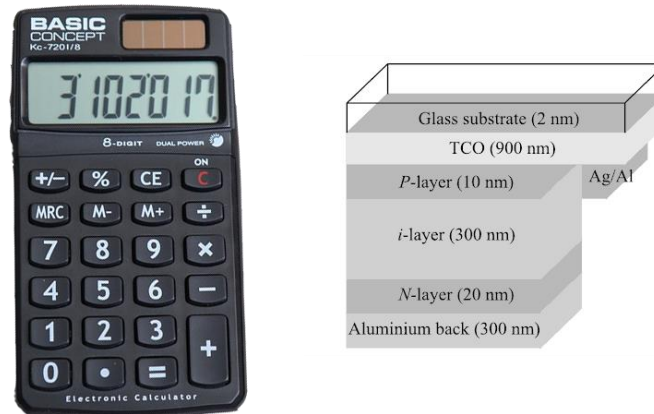
Figure 12. Left: a-Si powered calculator. Right: structure of a single junction a-Si solar cell in superstrate configuration. Sources: pixabay.com (right) and [55] (left).
