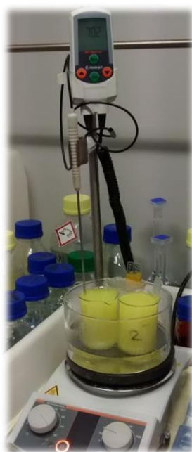
Figure 35. Setup for CdS chemical bath deposition.
