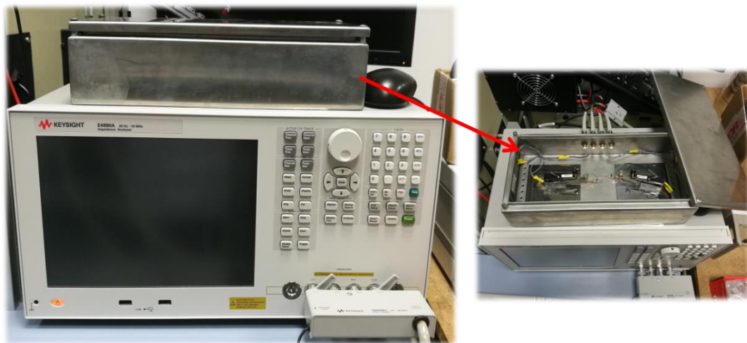
Figure 29. Keysight E4990A based capacitance-voltage measurement setup.
