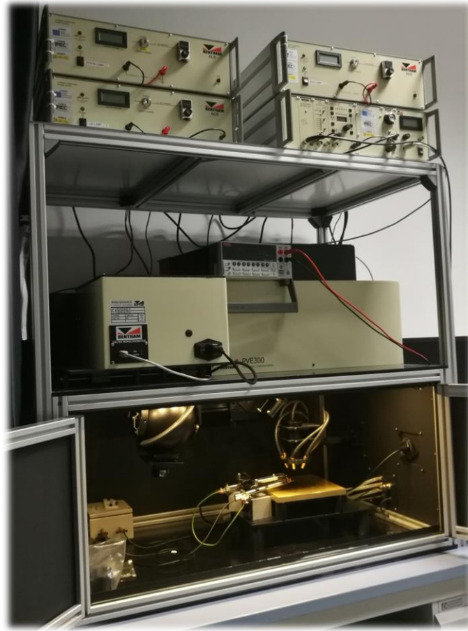
Figure 31. Spectral response system used for EQE measurements.
