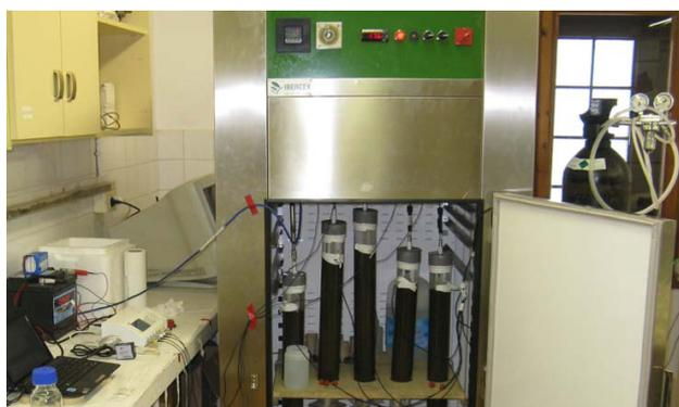
**Figure 2.** Experimental setup. The incubation chamber ensured dark and controlled temperature ( $\pm 1^\circ\text{C}$ ) conditions. Five intact lake sediment cores could be processed at once using their respective  $\text{N}_2\text{O}$  sensors.
