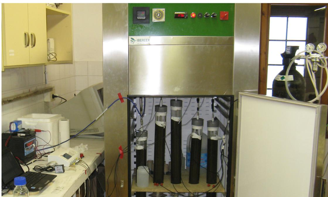
**Figure 5.2.** Experimental setup. The incubation chamber ensured dark and controlled temperature ( $\pm 1^\circ\text{C}$ ) conditions. Five intact lake sediment cores could be processed at once using their respective  $\text{N}_2\text{O}$  sensors.
