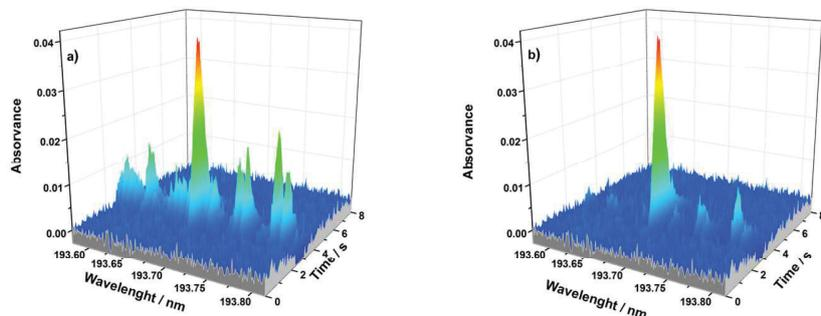
Fig. 4 Time-resolved absorbance spectrum in the vicinity of the 193.696 analytical line using SS-HR-CS GF AAS recorded for TORT-2 (a) without correction and (b) after correction using LSBC and  $\text{NH}_4\text{H}_2\text{PO}_4$  as a reference spectrum. In both cases  $15 \mu\text{g Pd} + 9 \mu\text{g Mg} + 0.06\%$  Triton X-100 was used as chemical modifier.  $T_{\text{pyr}} = 1200 \text{ }^\circ\text{C}$  and  $T_{\text{at}} = 2400 \text{ }^\circ\text{C}$ .
