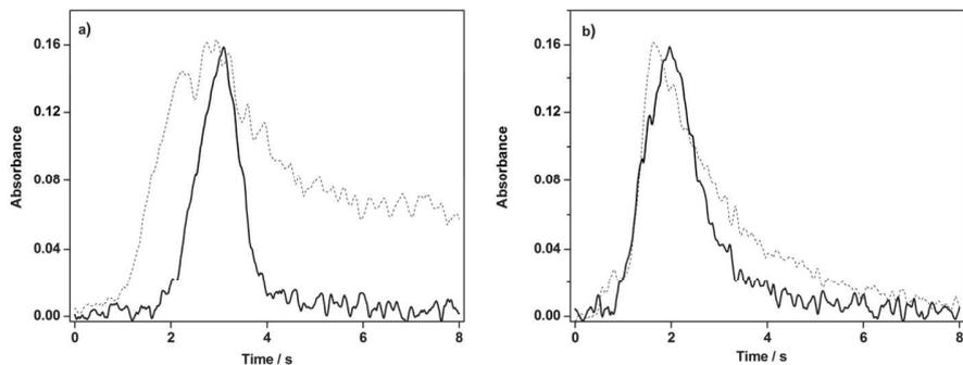
Fig. 2 Absorbance signals for As using SS-GF AAS. The solid lines represent atomic absorption and dotted lines represents the background signal. (a) Tort-2 (b) 1 ng As. Both in the presence of 15  $\mu\text{g}$  Pd + 9  $\mu\text{g}$  Mg + 0.06% (v/v) Triton X-100 as the chemical modifier.  $T_{\text{at}} = 2400$   $^{\circ}\text{C}$  and  $T_{\text{pyr}} = 1200$   $^{\circ}\text{C}$
