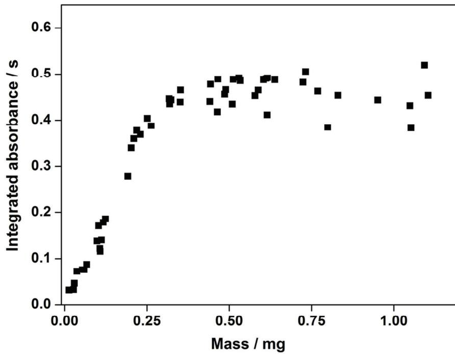
Fig. 3 Influence of the sample mass (TORT-2) on the integrated absorbance value using 15  $\mu\text{g}$  Pd + 9  $\mu\text{g}$  Mg + 0.06% (v/v) Triton X-100 as chemical modifier,  $T_{\text{pyr}} = 1,200$   $^{\circ}\text{C}$  and  $T_{\text{at}} = 2400$   $^{\circ}\text{C}$
