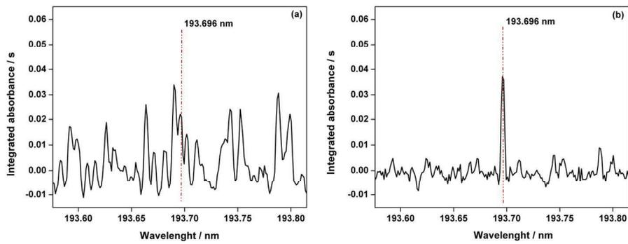
Fig. 5 Absorption spectra in the vicinity of the 193.696 nm analytical line for the CRM TORT-2 using SS-HR-CS GF AAS (a) without correction (b) after correction with LSBC using  $\text{NH}_4\text{H}_2\text{PO}_4$  as reference spectrum. In both cases  $15 \mu\text{g Pd} + 9 \mu\text{g Mg} + 0,06\%$  Triton X-100 was used as modifier and  $T_{\text{pyr}} = 1200 \text{ }^\circ\text{C}$  and  $T_{\text{at}} = 2400 \text{ }^\circ\text{C}$ .
