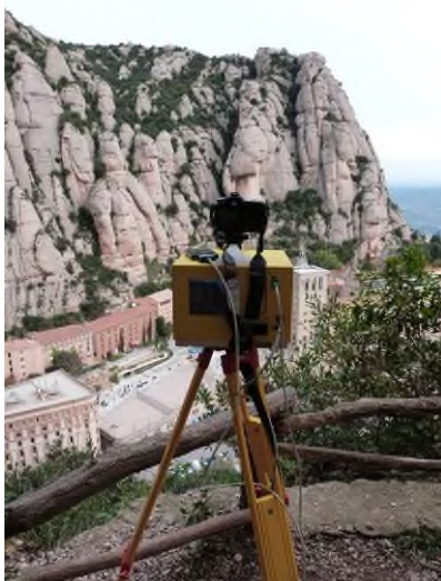
Figure 9. Data acquisition with the TLS equipment in Montserrat Monastery cliff.
