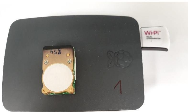
Figure 50 GSS Cozir LPTM NDIR  $CO_2$  sensor device
