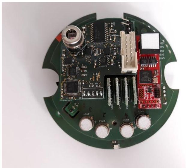
Figure 46 View of the sensors integrated into the Prototype 2
