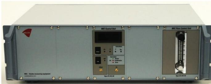
Figure 9. Picture of the Measuring Ionization Chamber EC-912 from Delta. The MIC was using during the fire and nuisance experiments performed at the standard fire room
