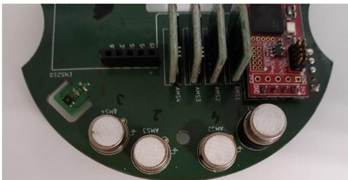
Figure 47 Metal Oxide sensors in the prototype 2
