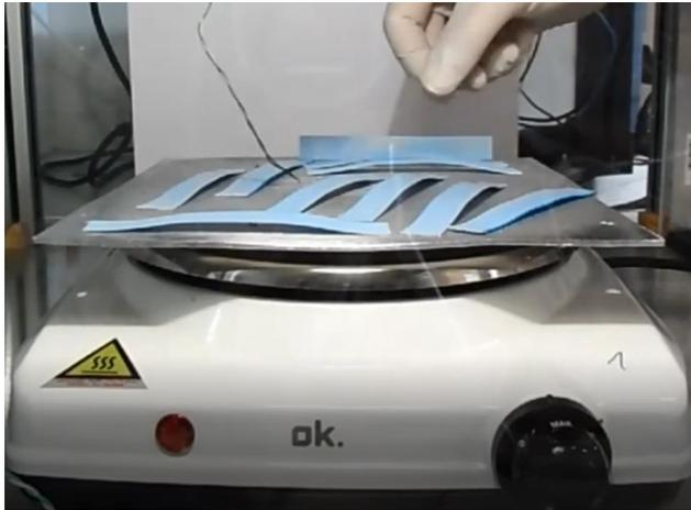
Figure 28 Picture of the Cable experiment performed at the chamber. Cable experiment consists of 10 pieces of flat cable of 10 cm and the fire is induced with the ignition of the wicks.
