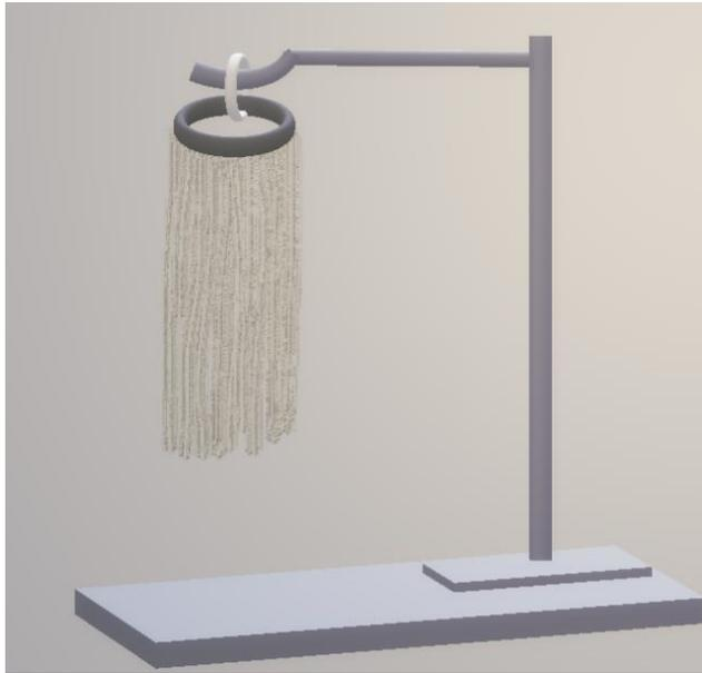
Figure 15 Illustration of the TF3 fire experiment performed in the fire room. The draw shows how the cotton wicks are hanged to the structure.
