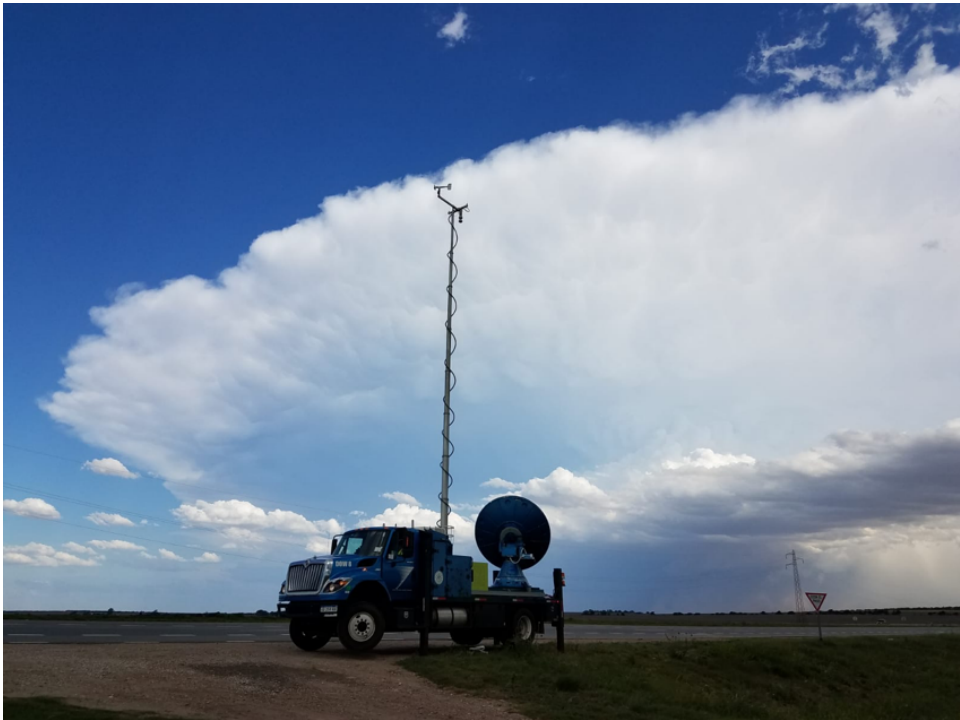
Figure A.4: DOW 8 scanning a supercell during one of the first IOPs. Author: McKenna W. Stanford
