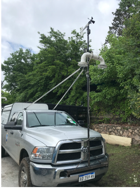
Figure A.2: Scout or Mesonet with anemometer on the front mast. Author: Anna del Moral
