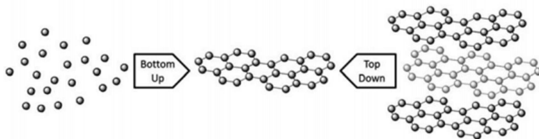
Figure 5. Both methods, top-down or bottom-up used to obtain 2D materials. Image adapted from reference Chaitoglou, S. Growth Study and Characterization of Single Layer Graphene Structures Deposited on Copper Substrate by Chemical Vapor Deposition.
