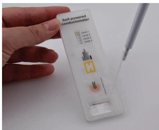
Figure 18. The final self-powered conductometer.
