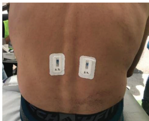
Figure 12. Image of two sweat absorbent patch attached to the lower back of volunteer at the end of the mountain race TRAIL PIRINEU 2019 while the sweat was being absorbed.
