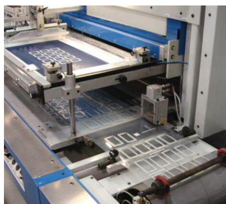
Figure 3. Roll-to-roll machine from Techprint Inc for screen-printing and lamination 13 .
