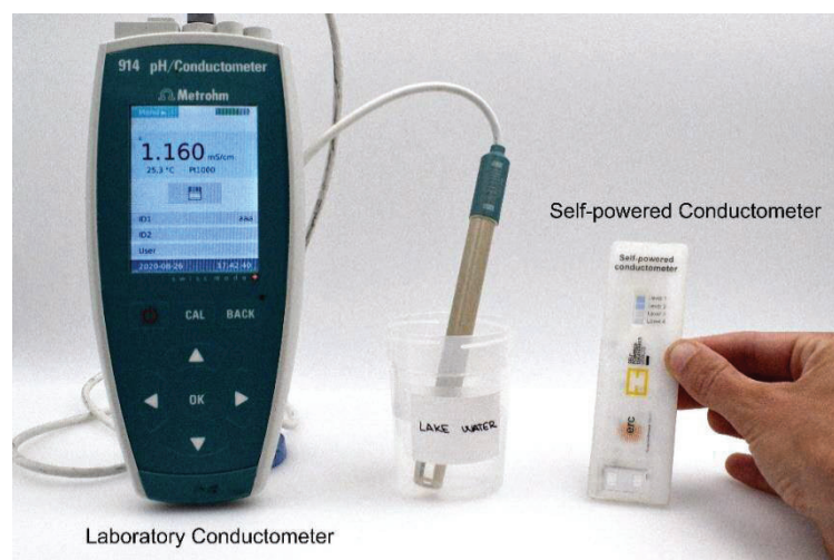
Figure 22. Image of the experimental setup used to compare the results obtained with a laboratory conductometer and the self-powered conductometer.
