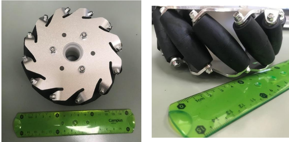
Figure 21. Different perspectives of the final solution for mecanum wheels. 15cm ruler for reference.
