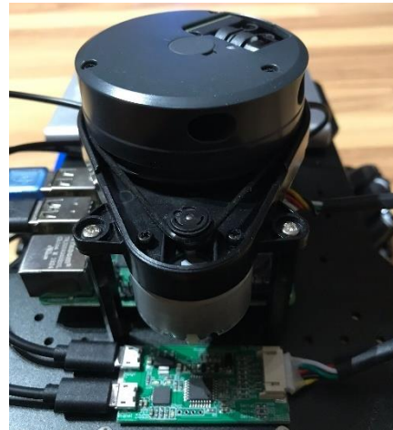
Figure 31. LIDAR fixed on small prototype.
