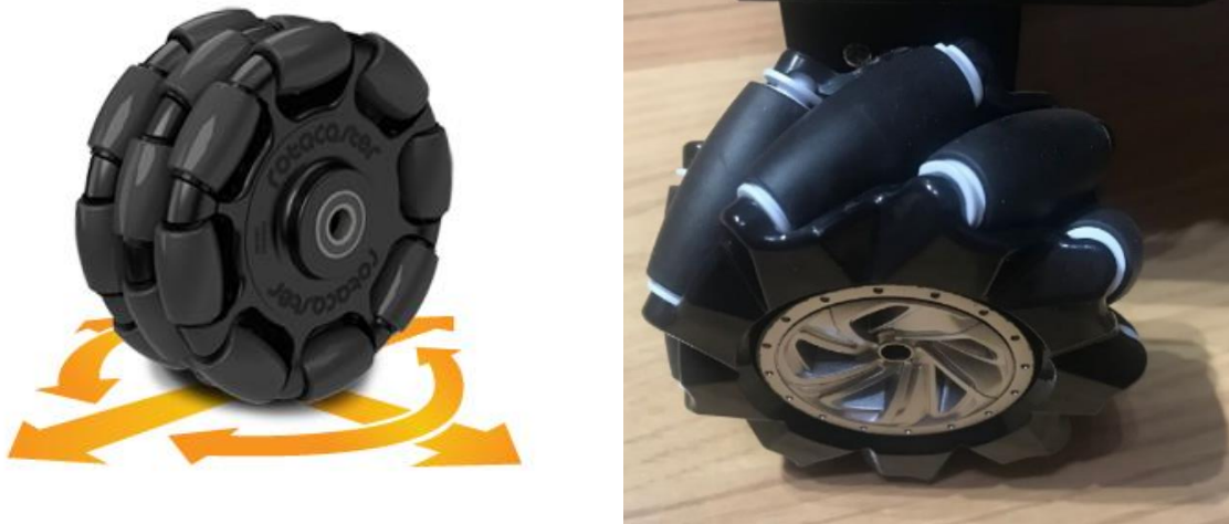
Figure 33. Omnidirectional wheels (Wikipedia, Omni wheel) (left) and mecanum wheels (right)
