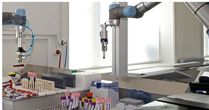
Figure 6. UR5 robots in a hospital lab carrying out automatized tasks.
