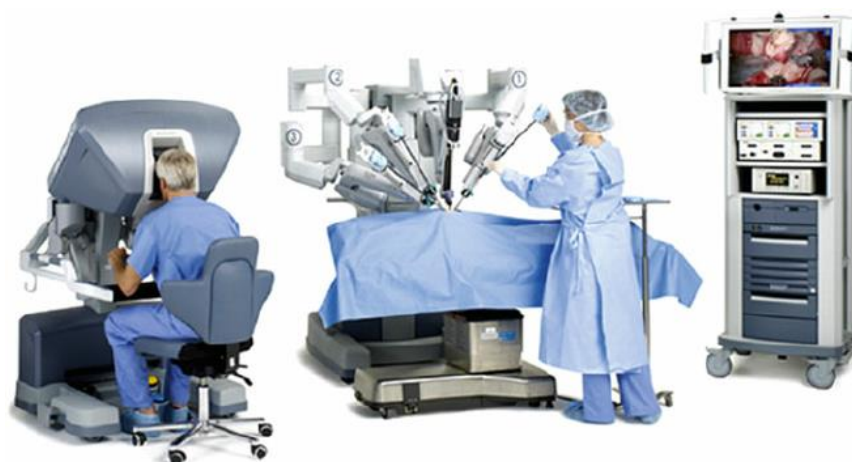
Figure 2. Da Vinci S set up components. In order: Surgeon's Console, the Surgical Cart and the Vision System.
