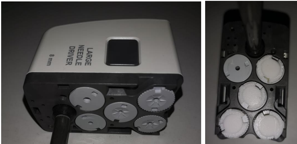
Figure 31. Mechanical solution to gear the servomotors with the EndoWrist disks.
