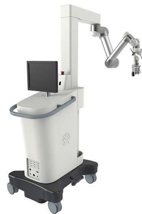
Figure 7. Modus V, from Synaptive Medical, coupled to a robot arm from Universal Robots.
