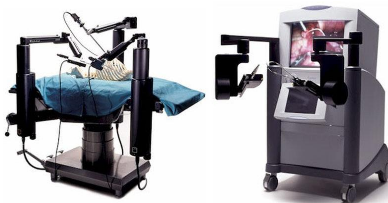
Figure 1. Zeus System components. Zeus Robot Arms in the left and the console in the right.
