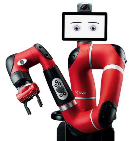
Figure 9. Sawyer robot from Rethink Robotics.
