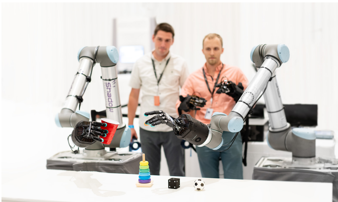
Figure 4. Application of the HaptX Gloves DK2 with a robotic arm. Extracted from: https://haptx.com/
