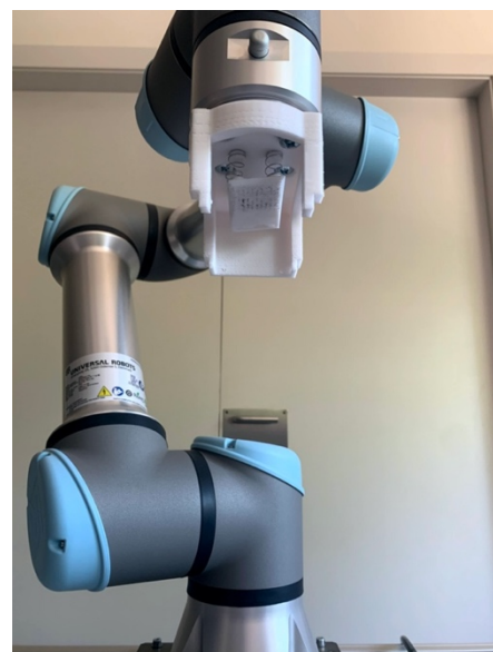
Figure 19. Component for the assembly of the UR5e to the EndoWrist tool. Made by the author of this document
