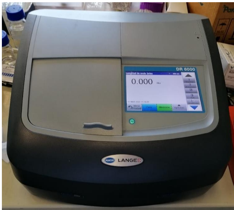
Figure 3.2. Spectrophotometer UV-Vis Hach Lange DR6000 employed in absorbance measurements.
