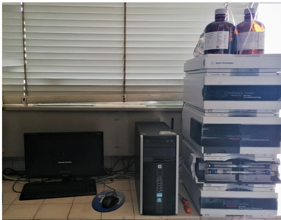
Figure 3.1. HPLC UV Infinity Series (Agilent Technologies) used for measuring the SMX residual concentration in solution.
