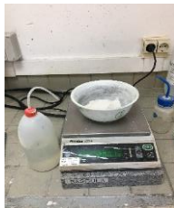
Figure 17: Flashing water bottle and mortar to determine the convenient amount of water.
