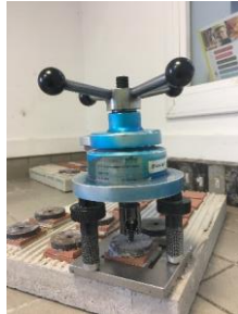
Figure 23: Pulling machine ready to pull up sufferers.).
