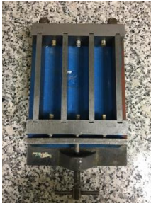
Figure 29: Standardized 4x4x16 cm molds for testing specimens.
