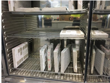
Figure 25: Oven at 70°C where slabs will remain during 14 days.
