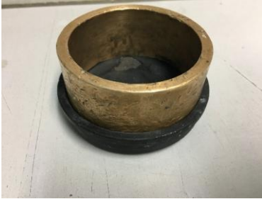
Figure 26: Round-shaped mold for the setting time test.
