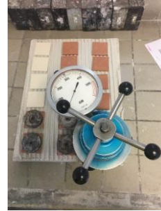
Figure 24: Top view of the slab and the pulling machine.
