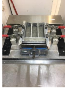
Figure 30: Vibrating instruments for levelling specimens.
