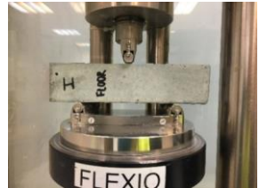
Figure 34: Flexural strength measurement.
