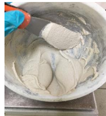
Figure 18: Fresh mortar mixed with the convenient amount of water.
