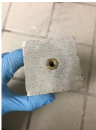
Figure 31: Testing specimen with nut.
