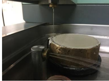
Figure 27: Round-shaped mold filled with testing mortar.
