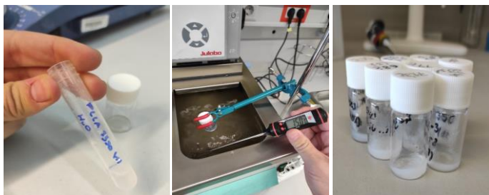
Figure 15. Hydrogel obtained by the mixture of enantiomeric PLA-PEG-PLA from micelle solutions.
