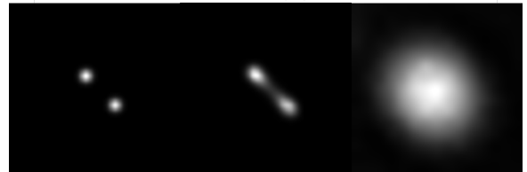
FIG. 9: Intensity profile of GT, SR image and EPI of the "Bibeads" zoomed image, from left to right order. 100nm distance between the centers of the points
