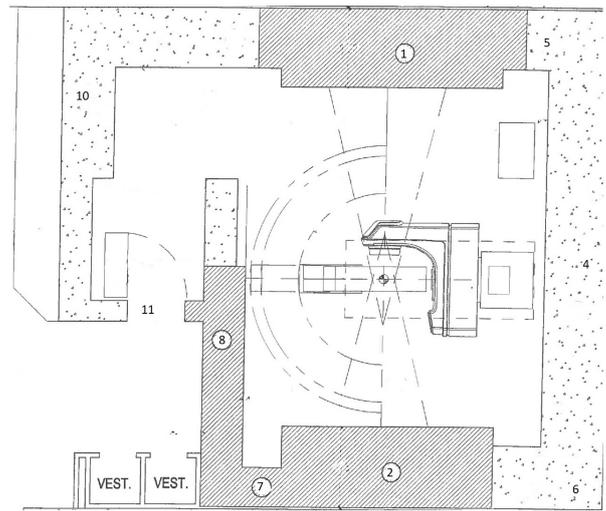
FIG. 2: Map of the accelerator bunker. The points 3 and 9 belong to the ceiling of the bunker.
