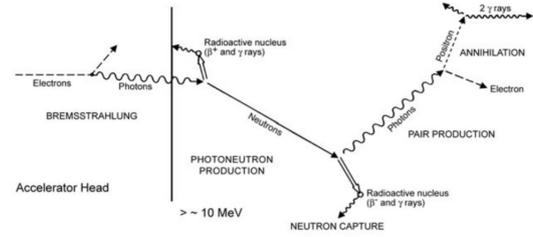
FIG. 1: Different radiation production reaction in an accelerator.
