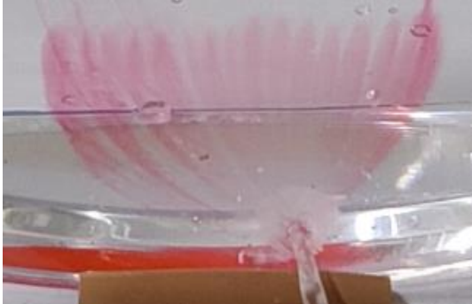
FIG. 3: A snapshots of the experiment where is easy to see streamlines in the surface surrounding S_2 , therefore, we conclude that there is a certain velocity in that region.
